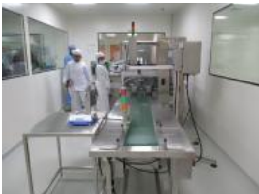
Blistering packing- ground floor.JPG
